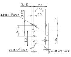
\*Please study & choose other appropriate hole diameters if confirmed the diameter values recommended above don't work with the soldering process.
