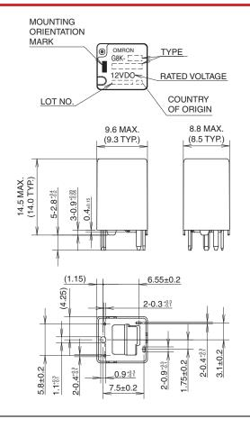
FOR REFERENCE: PCB MOUNTING HOLES (BOTTOM VIEW)
